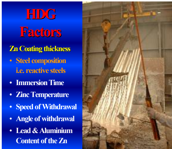
Hot Dip Galvanizing Process and factors that affect coating thickness
